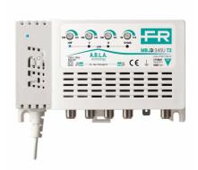
2-input (III+DAB, UHF) multiband TV indoor amplifier with 35dB gain and up to  $120dB\mu V$  output level on UHF band, separate amplification with independent level adjustment (20dB) for each input and low noise figure. T2 technology with UHF cut band for LTE 4G @790MHz and 5G @694MHz.
